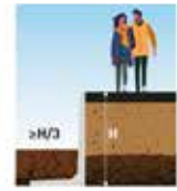
CLF10GSR uniform distributed overload 5 kN/m² no traffic, just pedestrians/cyclists
