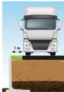
DLF10GSZ uniformly distributed overload 40 kN/m² at edge distance 1 m equivalent to load mode LM1 according to NBN EN 1991-2
