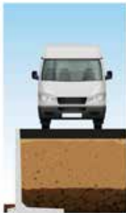
DLF10GSZ uniform distributed overload 25 kN/m²
