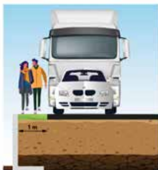
LVF RANGE heavy traffic, uniform distributed overload according to NBN EN 1991-2
