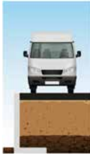
DLF10GS uniform distributed overload 25 kN/m²
