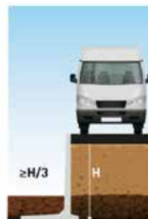
DLF10GSRZ uniform distributed overload 25 kN/m²
