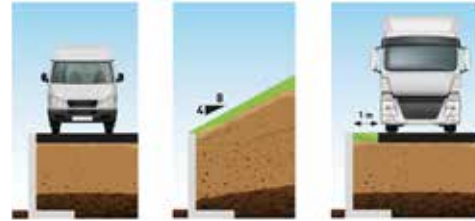
DLF10GS uniform distributed overload 25 kN/m²
